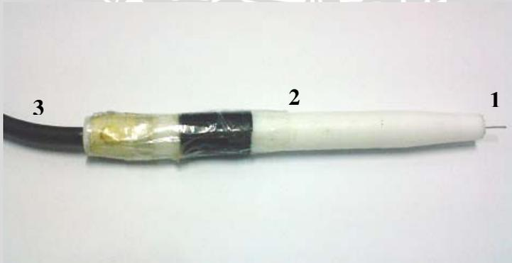
**Gambar 4.1** Konstruksi ESI nitrat tipe kawat terlapis
