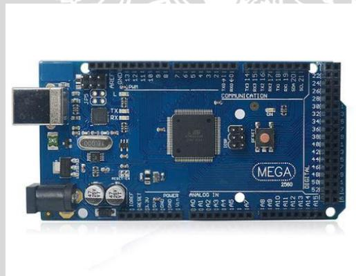
**Gambar 2.6** Arduino mega
