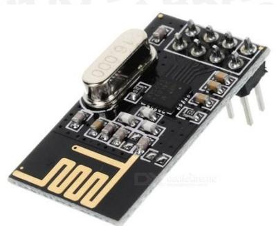
**Gambar 2.4 Wireless Module NRF24L01**
