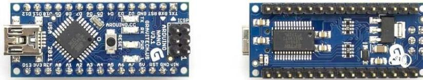
**Gambar 2.3 Arduino Nano v3.0**
