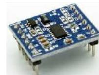
**Gambar 2.2 Sensor accelerometer MMA7361**
