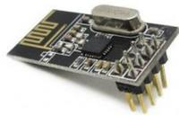
Gambar 2.4 Modul *transceiver* nRF24L01
