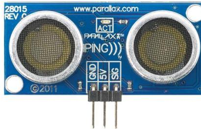
**Gambar 2.6 Sensor Ultrasonik (PING)**
