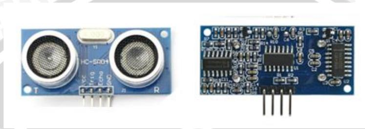
**Gambar 2.13** Sensor *Ultrasonic* HC-SR04
