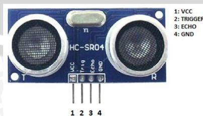
**Gambar 2.14** Pin Pada Sensor *Ultrasonic* HC-SR04
