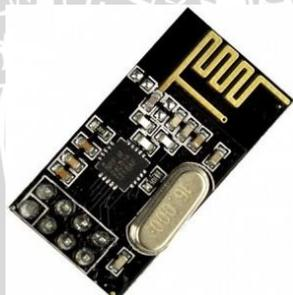
**Gambar 2.10 Modul nRF24L01**
