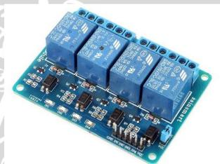
Gambar 4.1 Module relay 4 Channel
