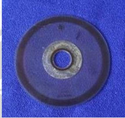
Gambar 2.18 Sensor *Timing Disk*
