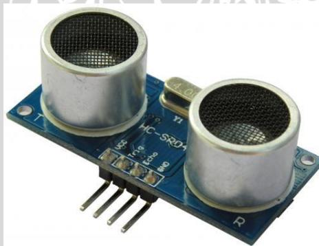
**Gambar 2.8 Sensor Ultrasonik**
