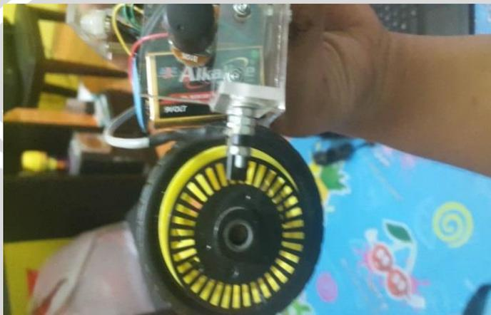
**Gambar 4.16 Pemasangan sensor *rotary encoder***
