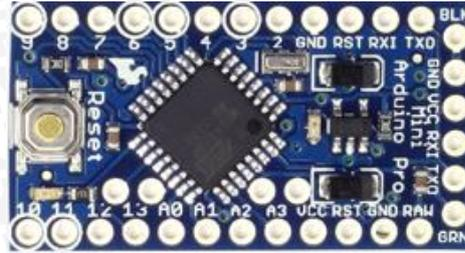
**Gambar 2.6 Board Arduino Pro Mini**
