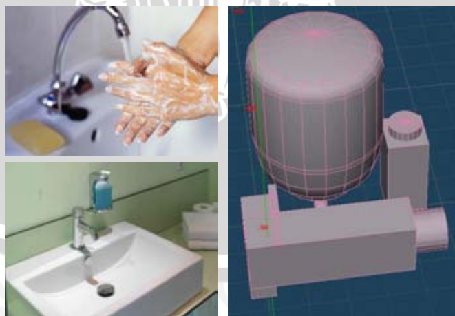
Gambar 4.7 Kran CTPS Build-in Sabun
