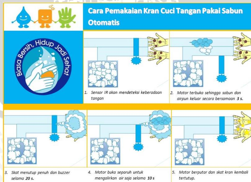
**Gambar 4.2 Skenario Sisi Alat**
