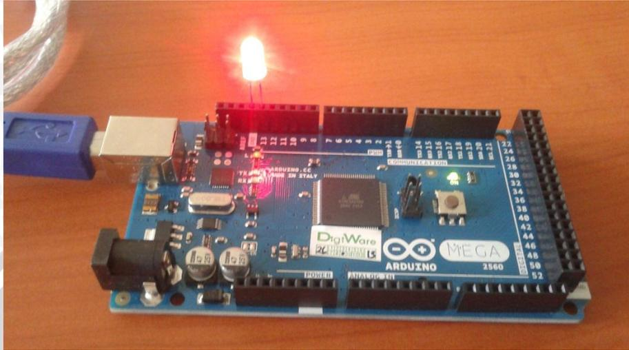
**Gambar 5.15** Mikrokontroler Arduino Atmega
