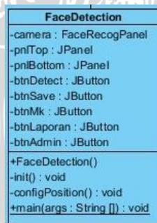
Gambar 4.5 Diagram Class *FaceDetection*
