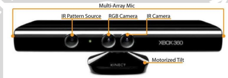
**Gambar 2. 2 Sensor Kinect**
