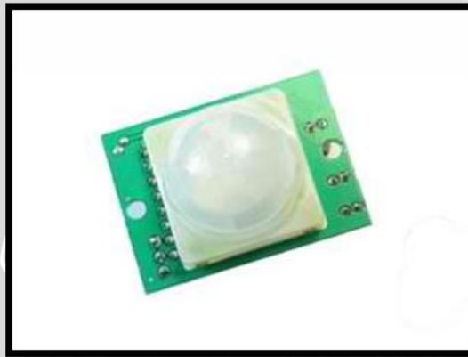
**Gambar 2.10** Sensor Gerak PIR
