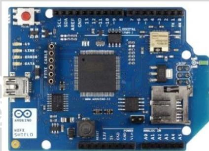
**Gambar 2.20**Arduino Wifi Shield
