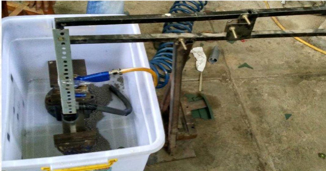
Gambar 3.6 Proses Shot peening
