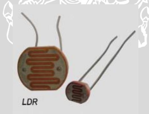
Gambar 2. 4 *Light Dependent Resistor*(LDR)
