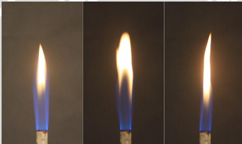
Gambar 4.16 Nyala Api minyak jarak non gliserol equivalence ratio 3,816
