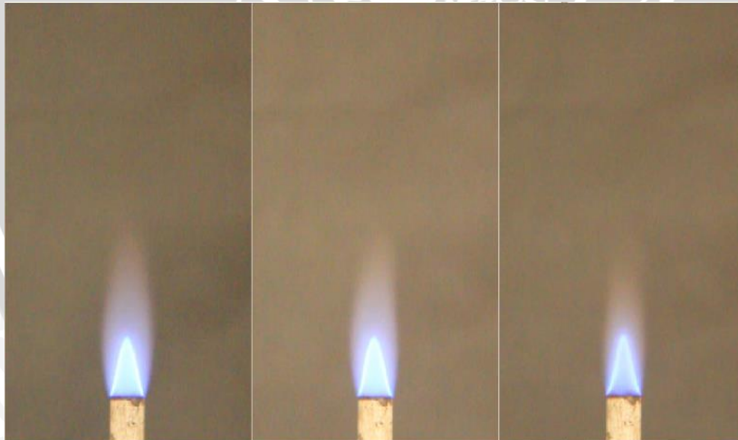
Gambar 4.11 Nyala Api minyak jarak non gliserol equivalence ratio 1,090
