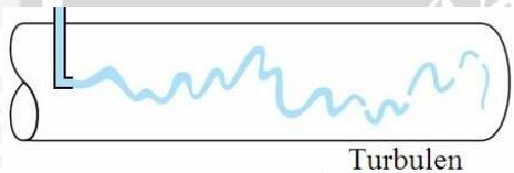
Gambar 2.4 Aliran turbulen
