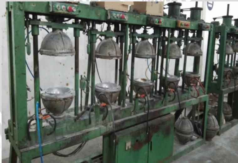
Gambar 4.19 Mesin *Vulcanizing Bladder*
