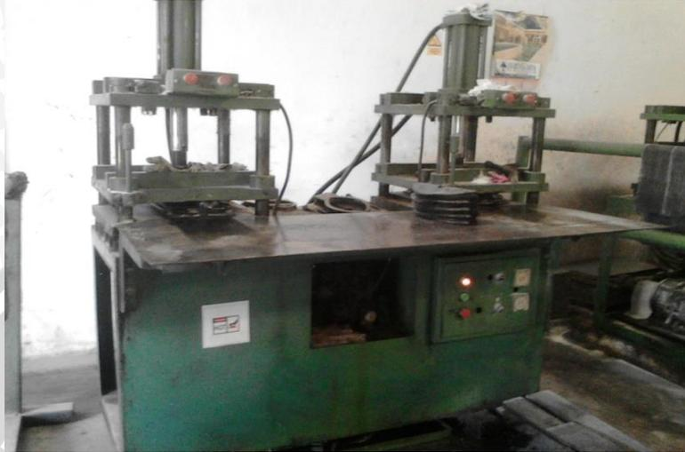
Gambar 4.18 Mesin *Cutting Sheet Bladder*
