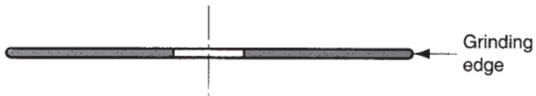
Gambar 2.13 *Abrasive Cutoff Wheel*
