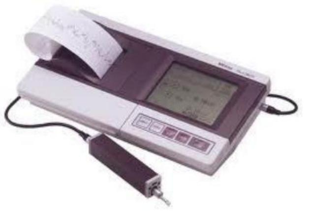
Gambar 2.23 *Surface Roughness Tester* Mitutoyo SJ-301
