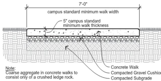
FIGURE 2.1: CAMPUS STANDARD SIDEWALK SECTION
