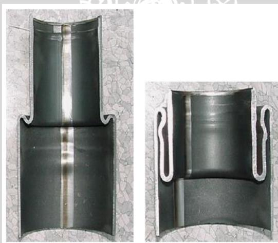
Gambar 2.1 Hasil Pengujian *Hydroformed Bumper Stays*
