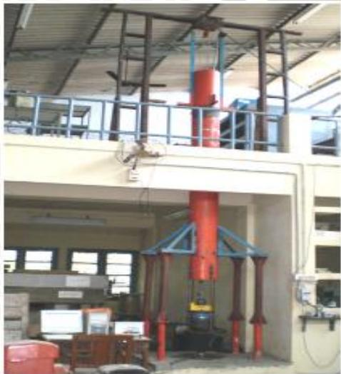
Gambar 2.12 Pengujian dinamis melalui *instrumented drop mass setup*
