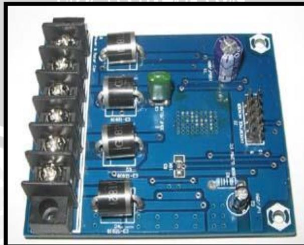
**Gambar 3.6 Driver Motor EMS 5A H-Bridge**
