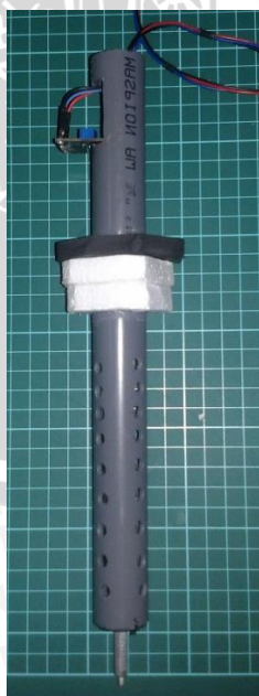
Gambar 4.5 Hasil Perancangan Sensor Salinitas Berbasis Sensor hall effect .
