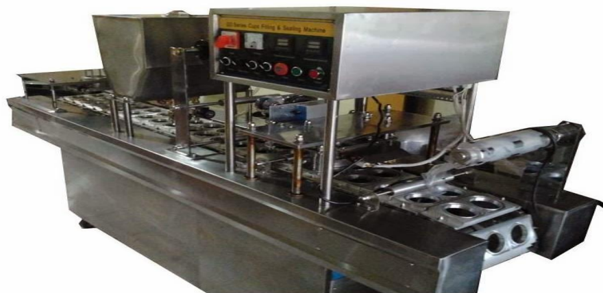
Gambar 1.1 Mesin Automatic Sealer Line-2
