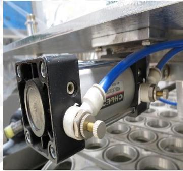
Gambar 4.7 Silinder *Pneumatic*
