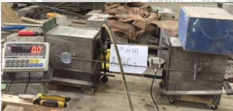
Gambar 4.2 Setting pengujian pull-out
