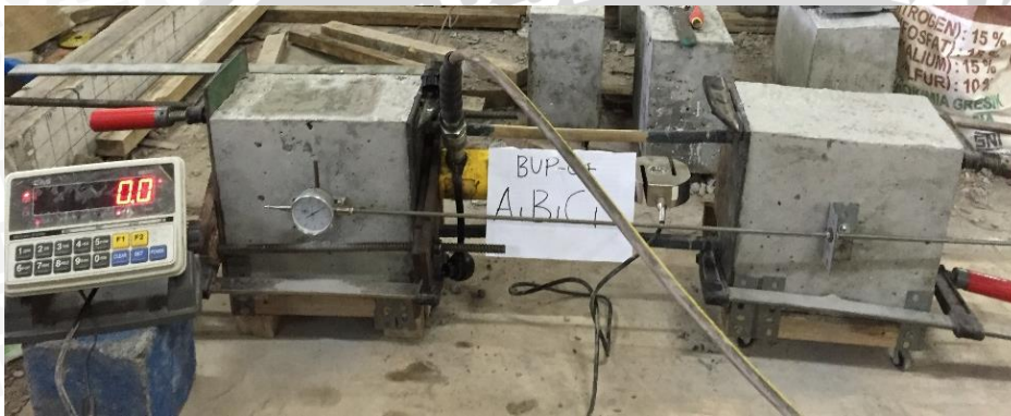
Gambar 4.4 Pengujian pull-out bambu
