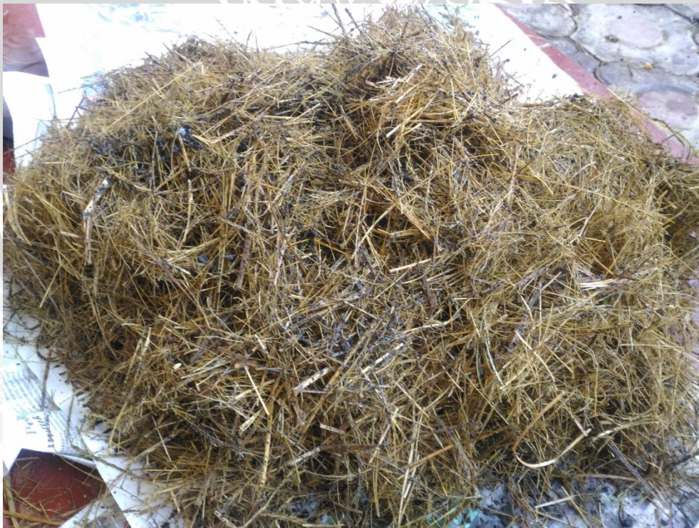
Gambar L5.6 Serat Bambu Dilapisi Pasir
