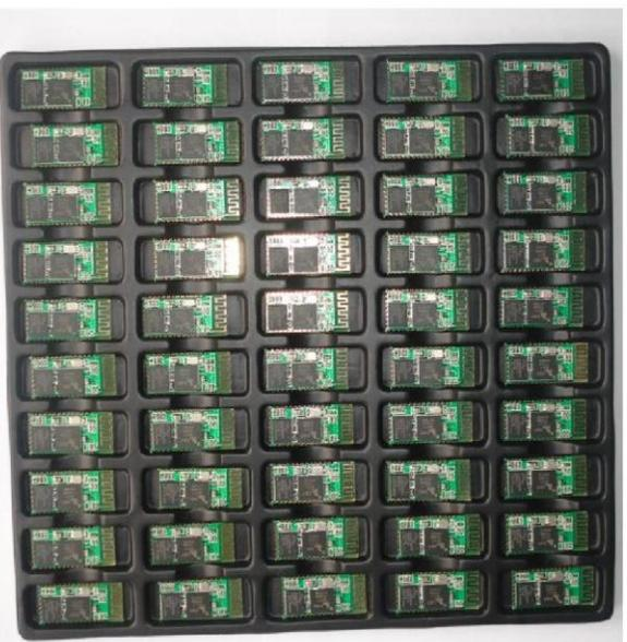
Figure 2 50 pieces chips in an anti-static blister package
