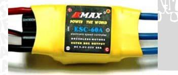
Low Voltage Protection Mode (Cutoff Mode) : power reducing / power cutoff, default is power reducing.
