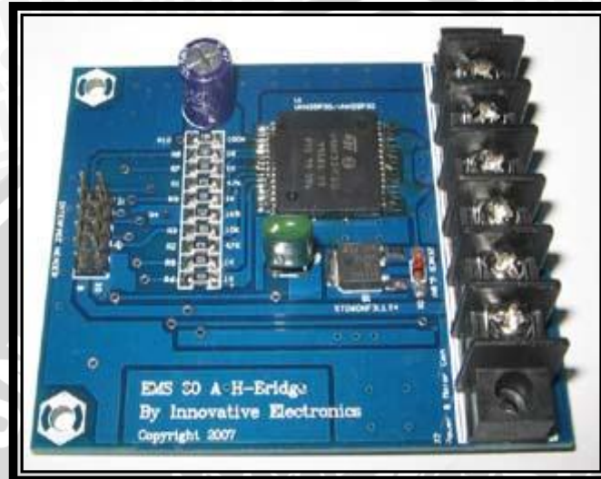
Gambar 4.5 Modul Rangkaian Driver EMS 30A H-Bridge ( www.Arduino.cc )
