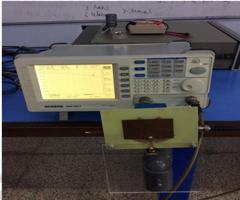
Pengukuran Return Loss Antena Single Patch
