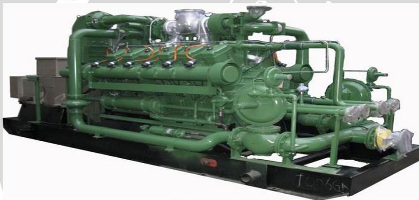
Gambar 2.9 Generator Set (GENSET) Biogas
