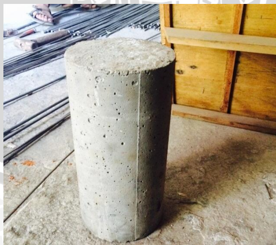
(a) Silinder Beton
