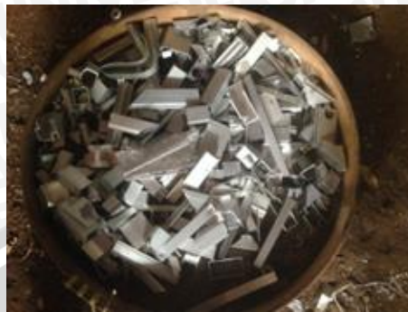
Gambar 3.8 Scrap Aluminium Al-Mg-Si Sumber: Laboraturium \alpha \beta \gamma Landungsari, Malang
