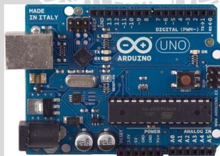
Gambar 4.4 Modul Arduino UNO (protostack.com)
