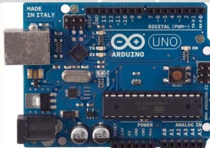
Gambar 2.8 ARDUINO UNO (Sumber: [protostack.com](http://protostack.com))
