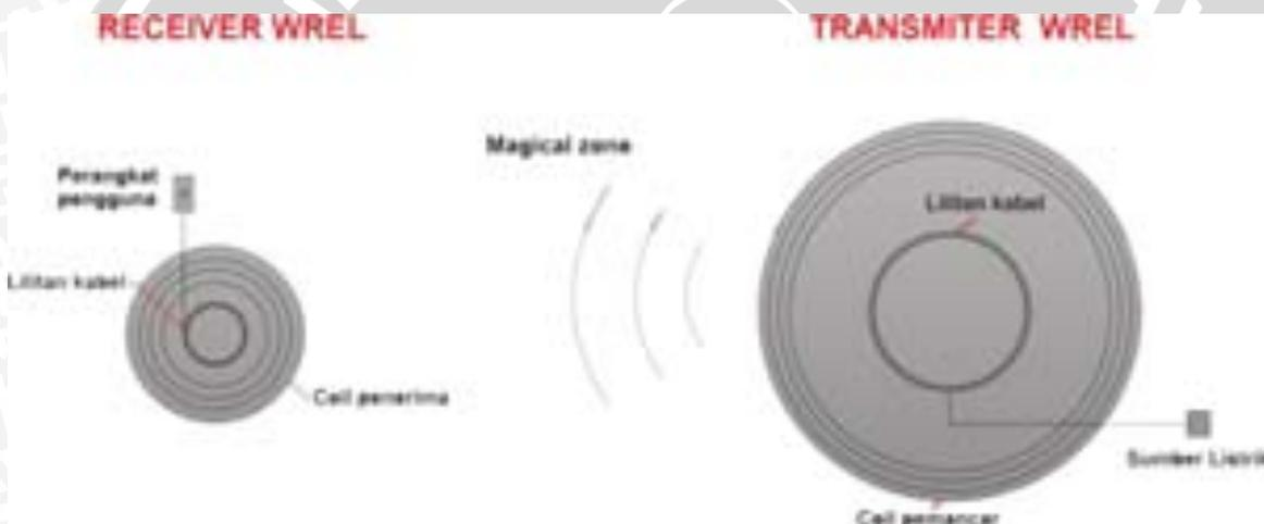
Gambar 4.68 Sistem listrik nirkabel (*wireless*)
