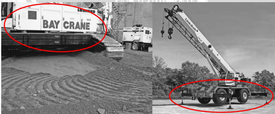
Gambar 4.6 Counterweight-based (kiri) dan outrigger-based (kanan) Sumber: Shapiro dan Shapiro (2010)
