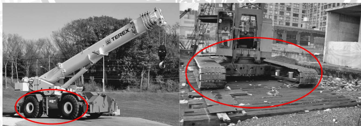
Gambar 4.5 Wheel-mounted (kiri) dan crawler-mounted (kanan) Sumber: Shapiro dan Shapiro (2010)
