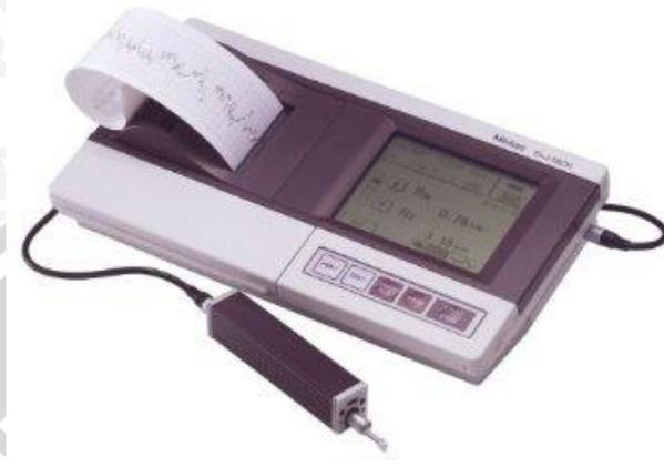
Gambar 2.16 *Surface Roughness tester* Mitutoyo SJ 301
