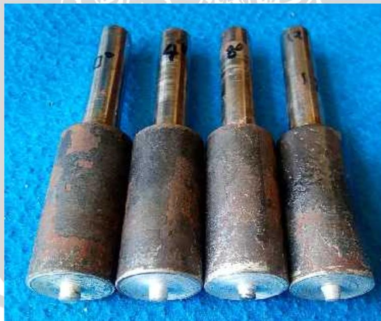
Gambar 3.4 *tool* pengelasan sudut  $0^{\circ}$ ,  $4^{\circ}$ ,  $8^{\circ}$ ,  $12^{\circ}$
