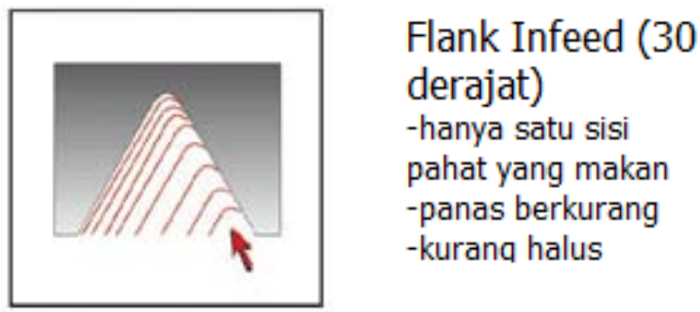
Gambar 2.4 Arah Flank Infeed
