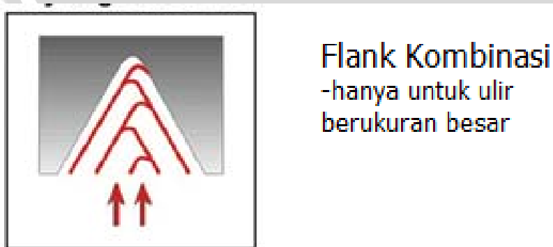
Gambar 2.5 Arah Incremental Infeed
