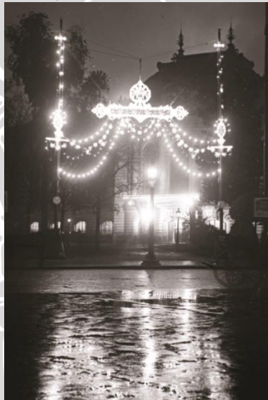
Gambar 2.22 Contoh Direct Sparkle dan Reflected Sparkle Sumber Gambar: Architectural Lighting: Designing with Light and Space
