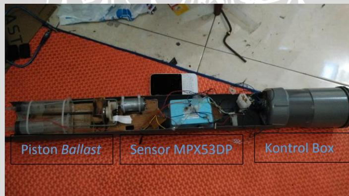
**Gambar 5. 2** Piston ballast, Sensor, dan kontrol box
