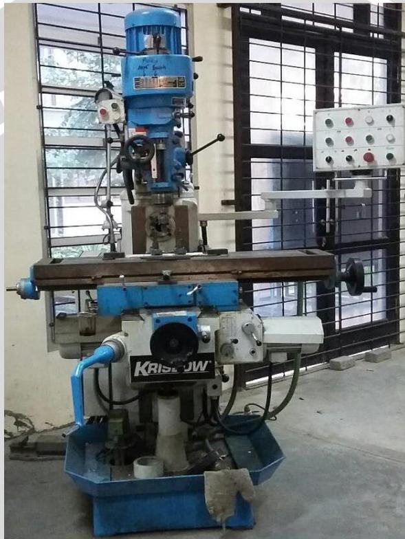
Gambar 3.2 Mesin *Milling Universal*
