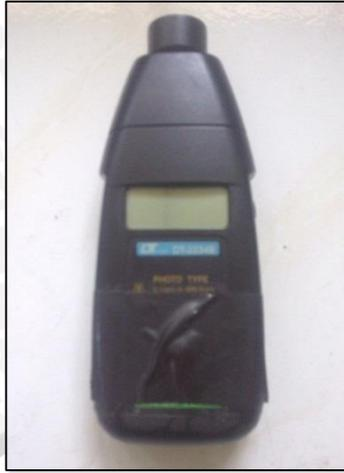
Gambar 3.3 *Digital Tachometer*
