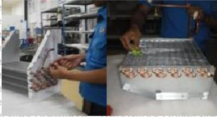
Gambar 4.5 Tube Assembling Process
